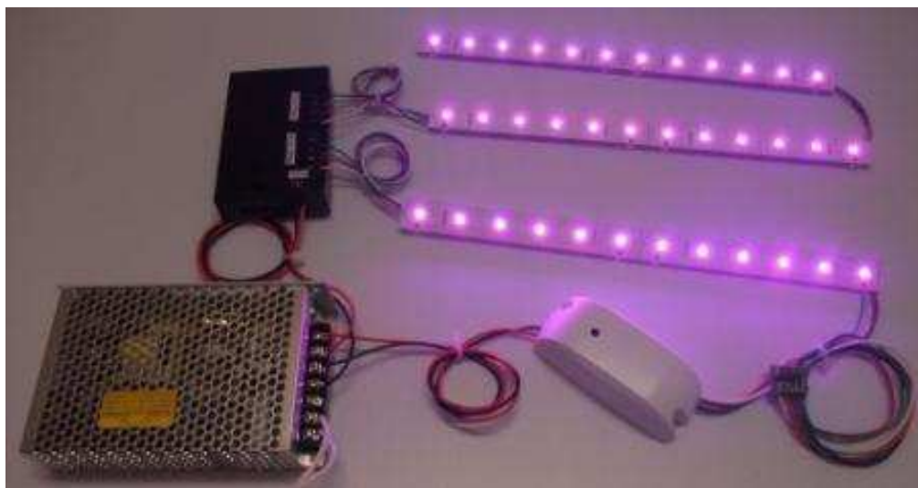
<AWCL-120-6P connects with the Signal repeater by lightings>
