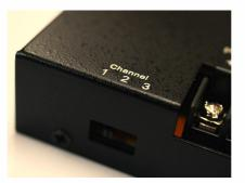
The switch to set channel 1~3.May use a IR remote controller to control the 3 groups of LED lighting
